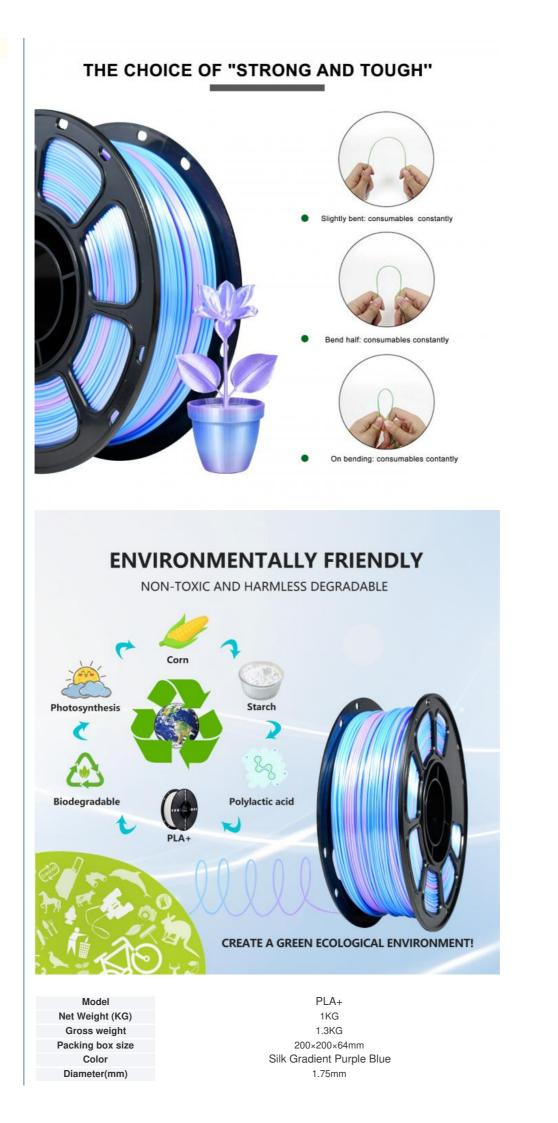
Tolerance(mm) Print Temperature (°C) Base plat Temperature (°C) Density Printing Speed Melt Index Bubble Length of Line (Ø 1.75±0.2mm) ±0.02mm 220-250°C 60°C 1.23±0.05g/cm3 40-100m 14-18g/10min (190°C,2.16kg) 100% without bubble
